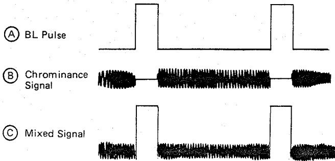
Fig. 87 White Balance Detector
