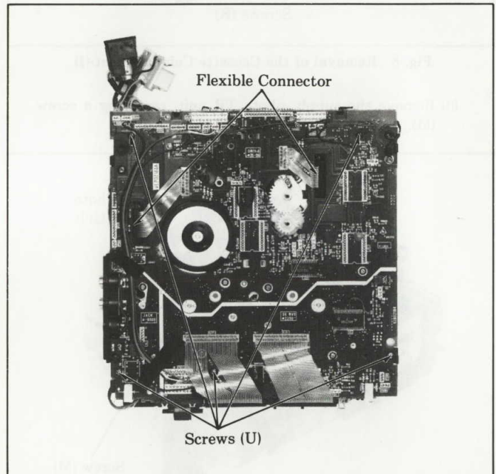
Fig. 16 Removal of Main C. Board-(1)
