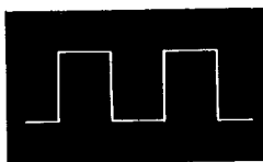
IC511 ① (H) 5.5Vpp IC511 ③ (H) 5.5Vpp
