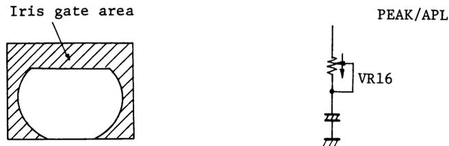
Iris detection of peak or APL may be predetermined by the PEAK/APL control (VR16). The iris is closed during CAL on, Bars on, or STANDBY mode.
